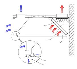
Section through canopy showing supply air system and the 3 stage canopy filtration.
