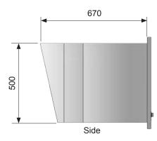
Each *Vortex Pod* will handle up to 1.2m³/s against a resistance of 150 Pascals and is powered by 240v 13 amp single phase supply.
